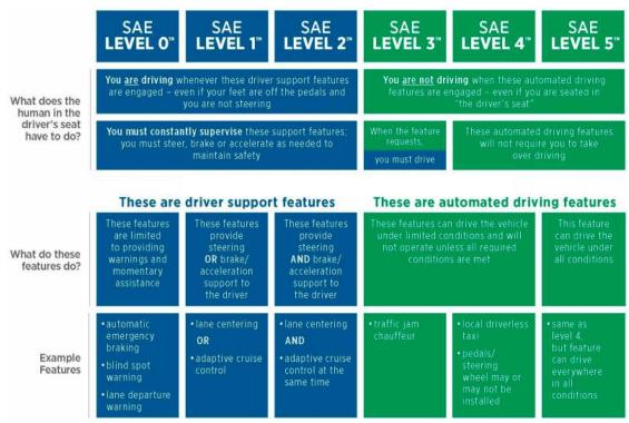
Figure 34 - Levels of driving automation84
